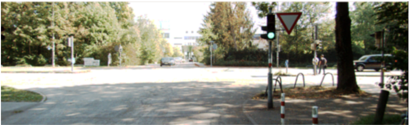
Figure 3: Equalised image using all channels at once (not recommended)
