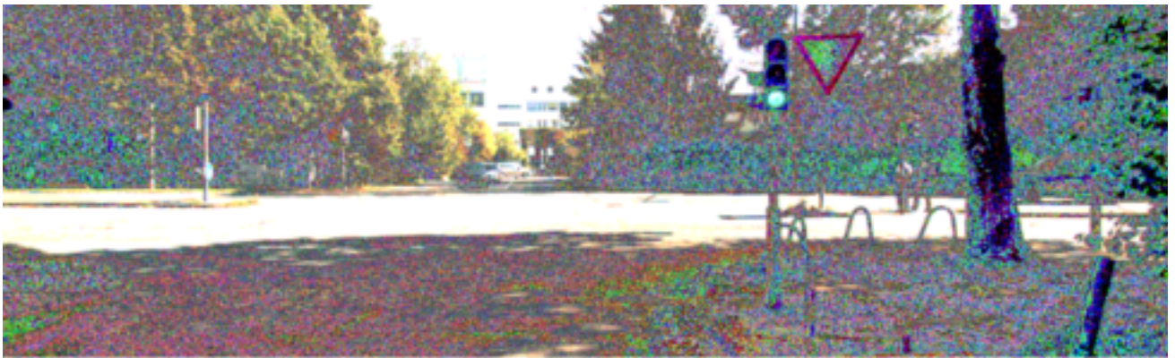
Figure 7: Image output with equalised RGB channels after splitting them (not recommended at all)
