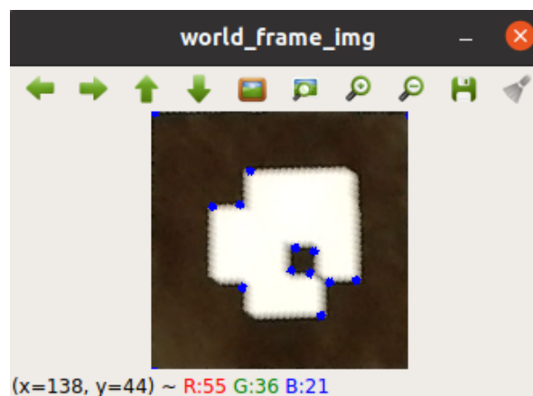
Figure 10: Warped image of the tag (Compensated the mirror image by dual warping)
