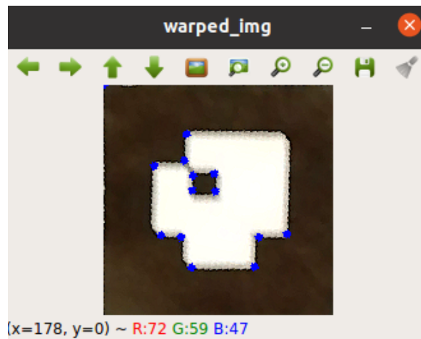
Figure 9: Warped image of the tag (Its the mirror image, which had to be compensated)
